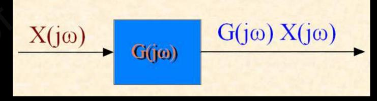
That is, doing  $s = 0 + j\omega$  in the transfer function G(s), one obtain  $G(j\omega)$
