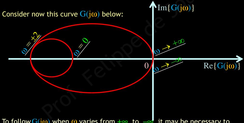
To follow  $G(j\omega)$  when  $\omega$  varies from  $+\infty$  to  $-\infty$ , it may be necessary to calculate *additional points* of  $\omega$  as in this Nyquist Plot above
