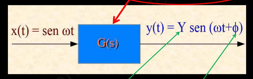
The output y(t) will have the same frequency of the input x(t), but, the amplitude Y and the phase angle  $\phi$ , will be, in general, different.
