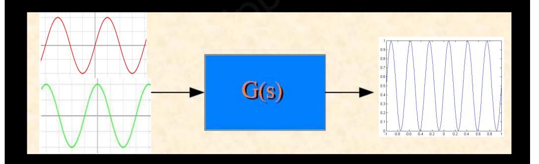
The advantage of these methods of analysis of systems by the frequency response is that they allow us to find both the absolute and relative stability of linear systems in closed loop only with the knowledge of frequency response in open loop, which can be experimentally obtained with signal generators (sinusoidal) and precision measurements instruments (both easily available in laboratory)
