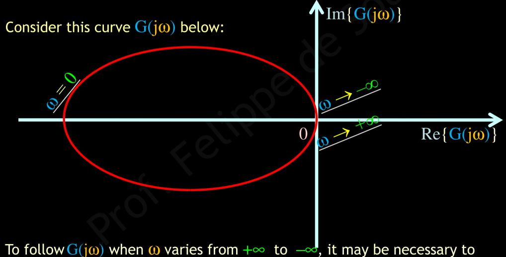
To follow  $G(j\omega)$  when  $\omega$  varies from  $+\infty$  to  $-\infty$ , it may be necessary to calculate *additional points* of  $\omega$  as in this Nyquist Plot above
