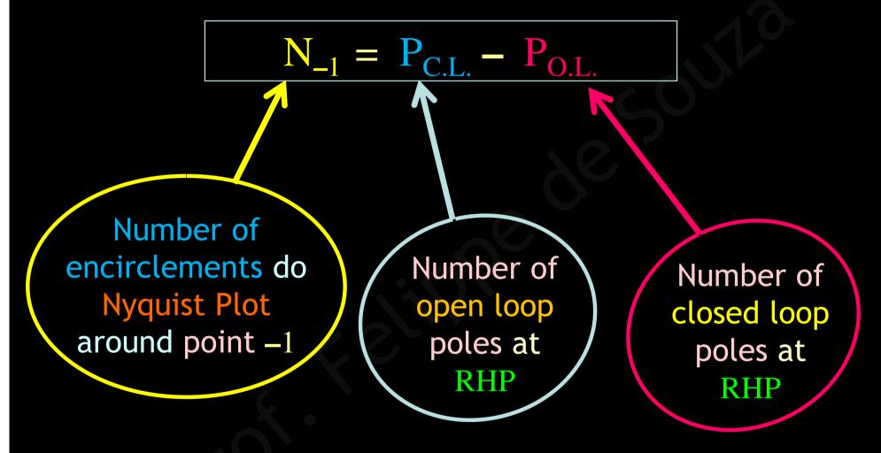
$N_{-1}$  = number of encirclements of  $G(j\omega)$  around point -1, which can be 'positive' (if direction is counter clockwise), or 'negative' (if direction is clockwise)
