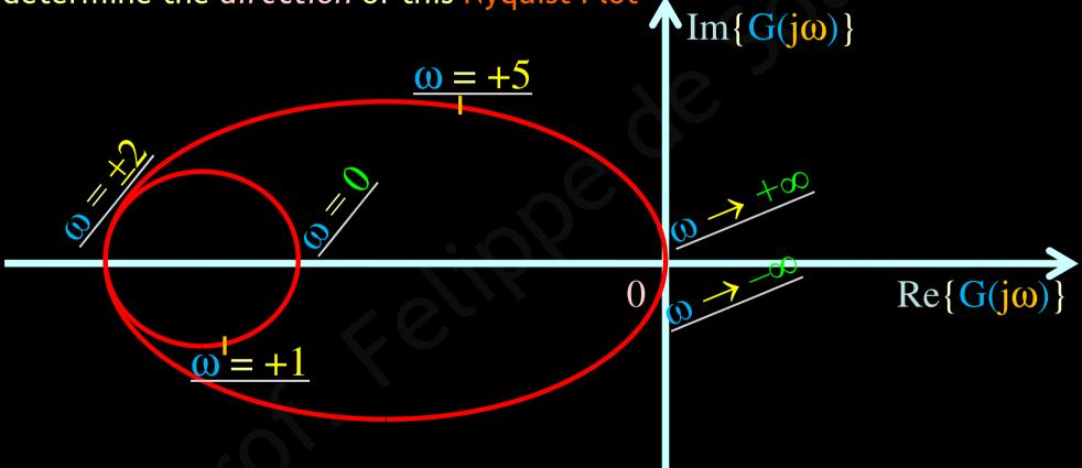
Calculating  $G(j\omega)$  for  $\underline{\omega} = \underline{5}$  and  $G(j\omega)$  for  $\underline{\omega} = \underline{1}$  we can write down the points G(j5) and G(j1) in the Nyquist Plot above
