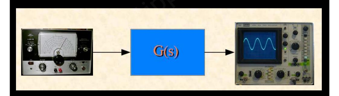
Therefore, the analysis of complicated systems can be done through tests of *frequency response* without being necessary to determine the *roots* of the characteristic equation (i.e., the *poles* of the *system*)
