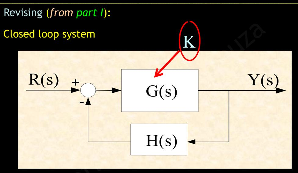
The "<u>Root Locus</u>" the locus of the poles of the closed loop system, when we vary the value of K
