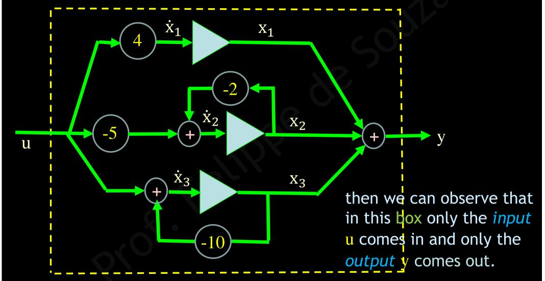
The variables  $x_1$  and  $x_2$  which stayed inside the box are part of an *internal* representation of the system, though its state variable.
