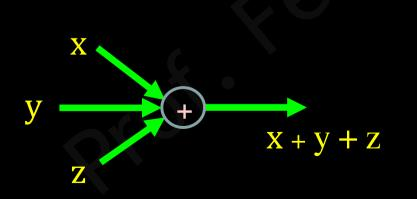
sums the input signals giving an output signal
