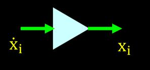
transforms an input signal  $\dot{x}_i$  in  $x_i$  in its output, that is, it integrates
