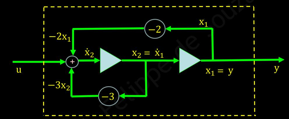
we can observe that in this box only the *input* **u** comes in and only the *output* **y** comes out.
