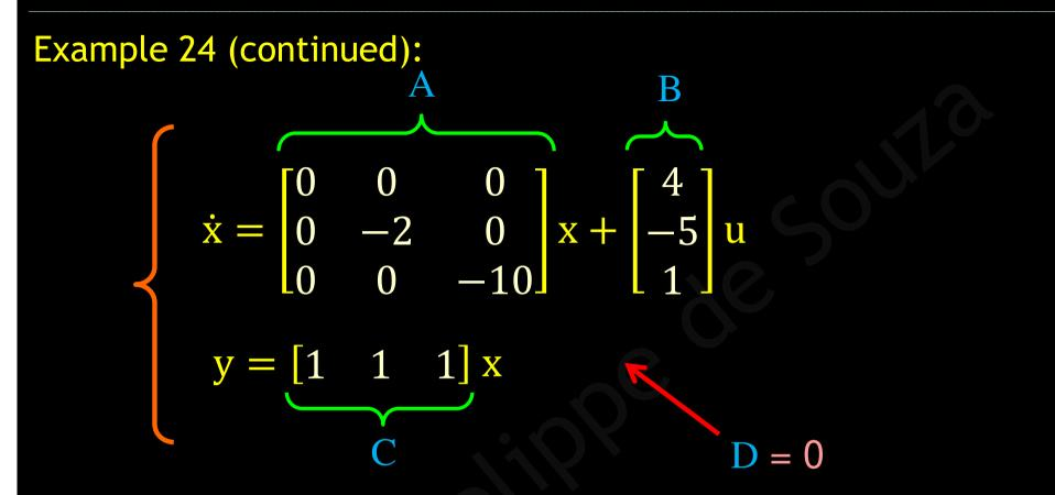
Note that *matrix* A is in the diagonal form in this *representation* and the *poles* of the system (s = 0, s = -2 and s = -10) are the elements of the *main diagonal*
