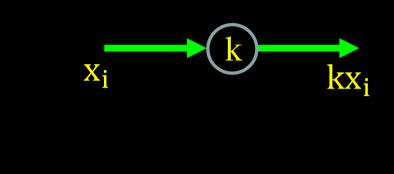
multiplies the *input* signal  $x_i$ by k, giving back  $kx_i$  in its *output*
