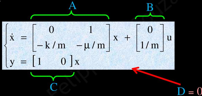
which is the *representation* of the system in *state equations*.
