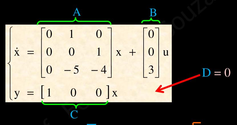
For the new *state variable*  $\overline{x}$  be the same as the old x, only changing the third component  $x_3$  by the double:  $\overline{x_3} = 2 \ x_3$ , the choice of  $\overline{P}$  should be:
