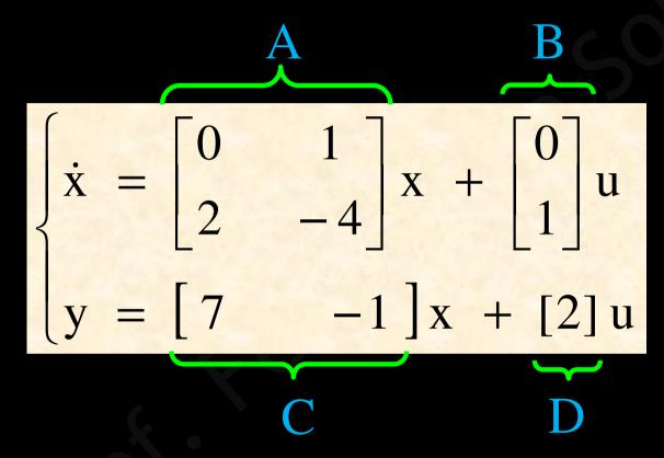
To calculate the *transfer* function, first we find the matrix (s I - A)
