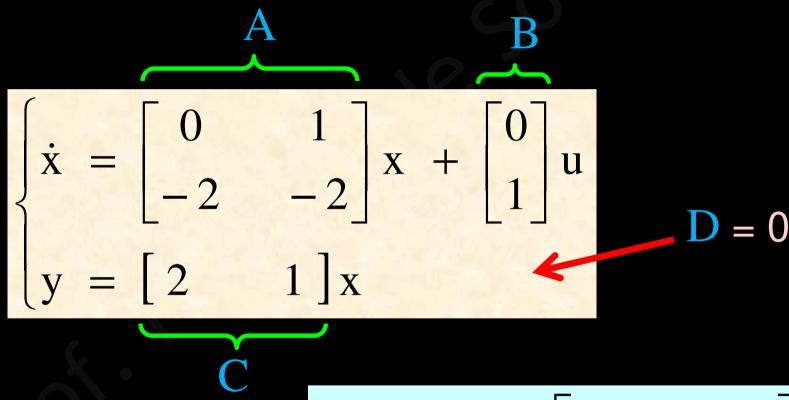
To calculate the *transfer* function, first we find the matrix (s I - A)
