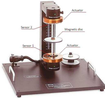
Fig. 1. Magnetic Levitation System made by ECP.
