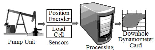
Figure 3. Data acquisition and signal processing.
