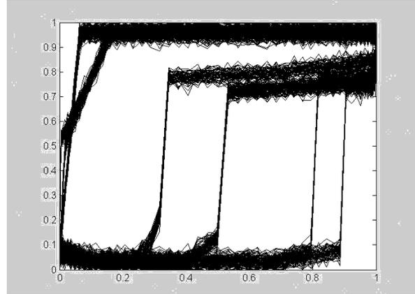
Figure 7. Set of artificial standards for cards with fluid pound.
