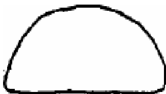
6-Leaking traveling valve
